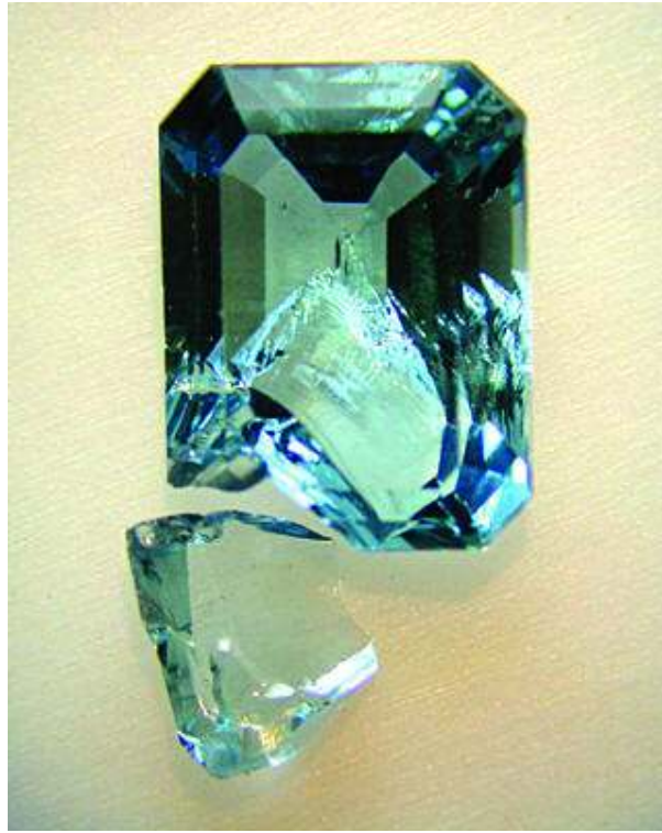
This topaz was damaged when moderate pressure was applied to a small cleavage. photo courtesy of Anton Nash.
