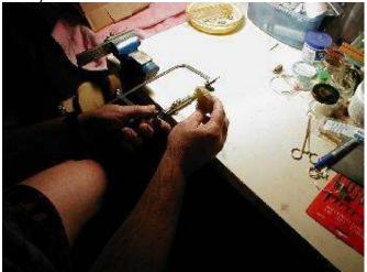
2. If your saw already has a blade in it, unscrew one side of the saw to release one end of the blade. Slip the coil onto the blade, and then secure the end of the blade back into the saw.
