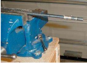
6. Pull the coil of wire off the bit and prepare for sawing the rings.
