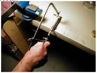
3. Now set the coil (which you just inserted onto the blade) into jump ring side of the jig. The cool part of this tool is that it has a place for the rings to just sit in place so you don't have to worry about the coil moving around in your fingers. You still need to hold the coil, but it moves much less. (If you check the Rio Grande tool catalog, you'll see some good, up-close pictures of both jigs.)
