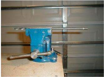
2. Now start with at least a foot or two of wire, and use the vice grips to hold the wire up against the bit.
