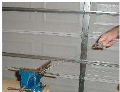
4. Hold the vice grips attached to the end of the wire, and wrap the wire evenly around the bit.
