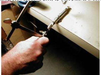
4. Line up the blade so it's in the middle of the coil and rest the blade into the grooves which are on either end of your coil. This is great because it helps you keep your sawing straight.
