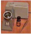
Another required tool for gemologists is the refractometer. A small drop of liquid with a high refractive index (RI) is placed on a glass cylinder in the top of the refractometer and illuminated from a separate light source (sometimes white light, but a monochromatic light source provides better accuracy). The RI is then read from a magnified gauge on the front of the refractometer.
