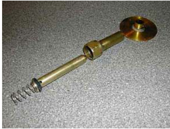
Injector Nozzle Dismantled
