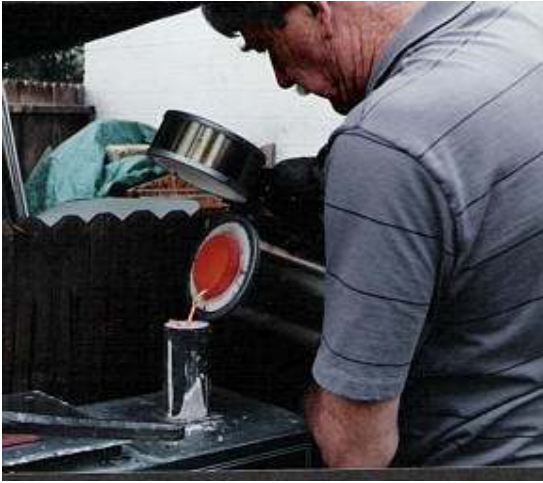
5. Metal is poured.
