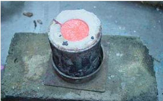
6. The hot flask is placed in the base assembly on the wax
