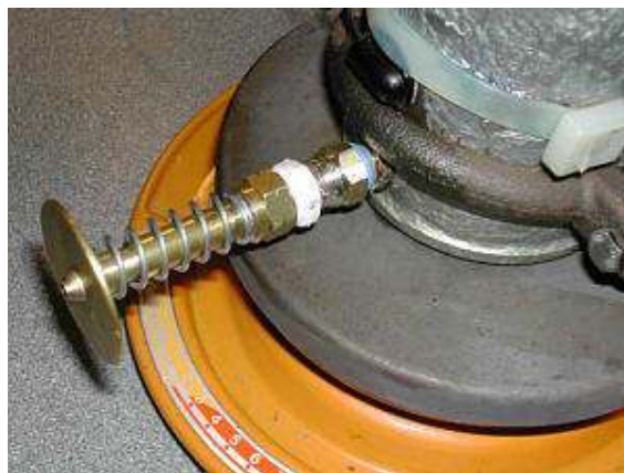
An Alternative External Spring Arrangement for the Injector Valve
