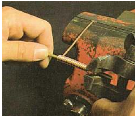
P4-3. Winding an oval coil
