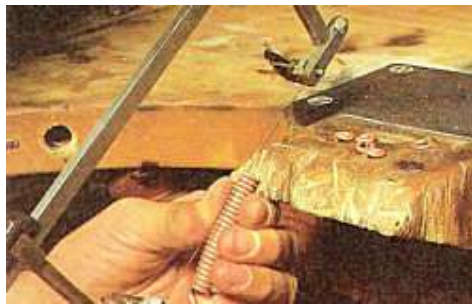
P4-5. Sawing off the links
