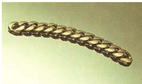
P4-11. Finished twisted curb chain
