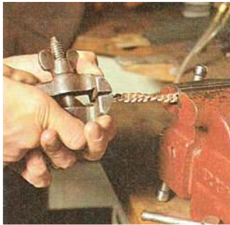
P4-9. Twisting the curb chain
