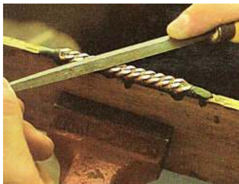
P4-10. Filing the facets of the chain while mounted on a dop stick
