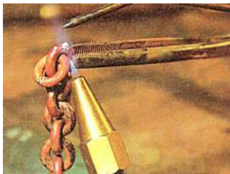
P4-8. Assembling and soldering the chain
