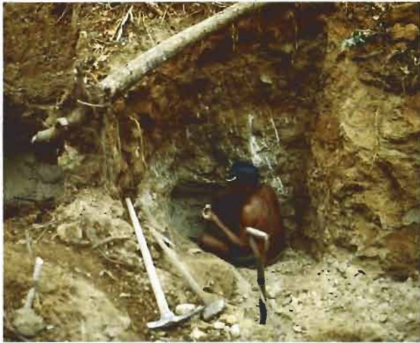
Figure 15. After only a meter of tunneling, this garimpeiro has reached the primary pegmatite (note the white feldspar) at Frade.
