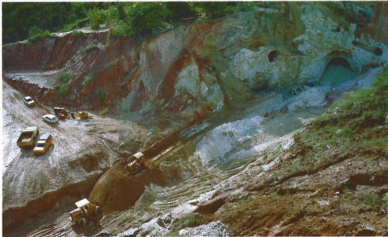
Figure 5. Heavy machinery is often required for hard-rock mining in Brazil. At the Golconda tourmaline mine, bulldozers are used to move the overburden and waste from the mine entrance.
