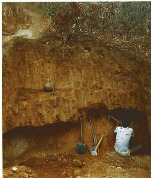
Figure 6. Pick and shovel are the basic tools of the garimpeiro searching for aquamarine crystals in the “soft rock” of this colluvial pit near the bottom of Frade valley.
