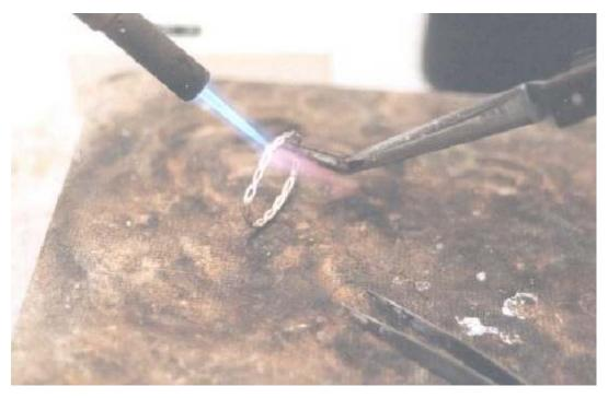
Soldering showing the use of the inner blue flame tip for maximum heat.
